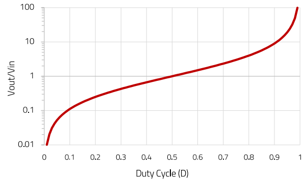
Figure 7: Ideal voltage conversion ratio of SEPIC
