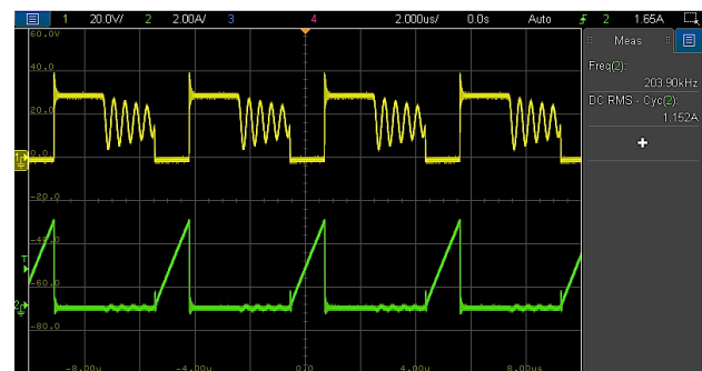
Figure 26: Measured Q_1 waveforms of DCM-SEPIC ( V_{Q1} (I), I_{Q1} (I))
